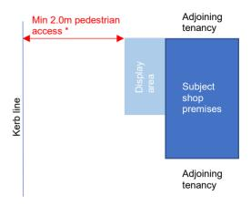
The plan for storage or display on a footpath area must be to scale and with clearly marked dimensions, showing:
